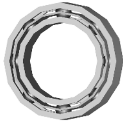
Fig. 4. Animation of the ball bearing model.
